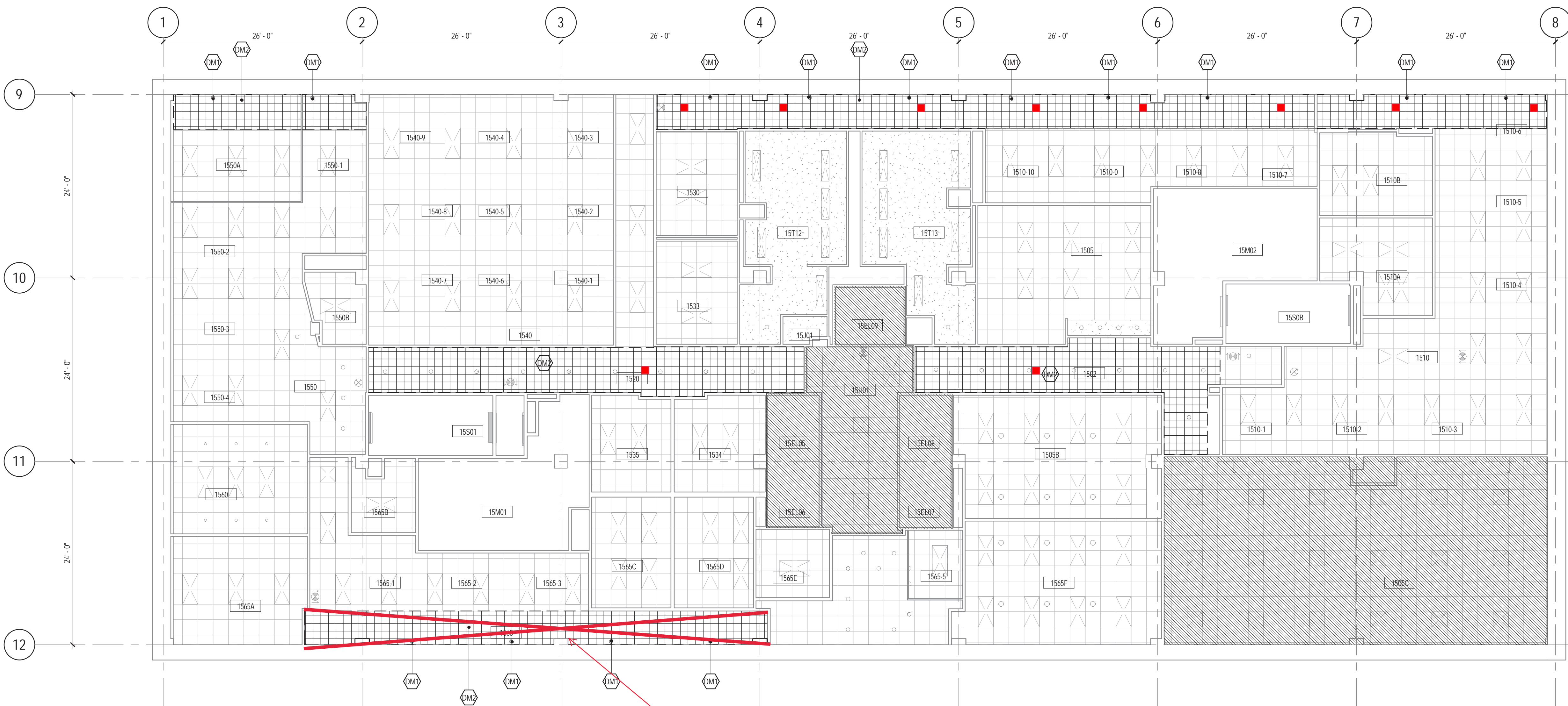
2 REFLECTED CEILING PLAN - LEVEL 15 1/8" = 1'-0"
